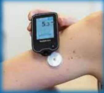
Freestyle Libre 2 scan or 'flash' the sensor with smartphone or receiver
